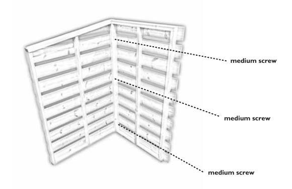
Step 2: Attach the blank with pilot holes to the left to the back using 3 medium screws and the top and bottom bar using 4 large srews.
