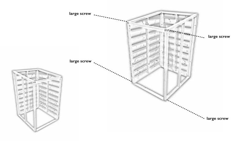
Repeat step 2 to make another side for the right side using the blank with pilot holes to the right.
