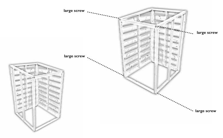
Repeat step 2 to make another side for the right side using the blank with pilot holes.
